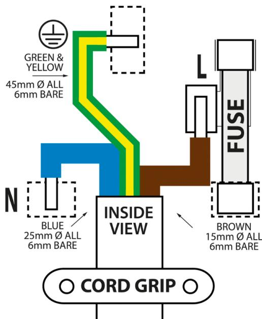
Fuses must be replaced with the same rating as the original; please refer to the fuse rating stated on the plug for this information. Only genuine fuses compliant with BS 1362 should be used.
